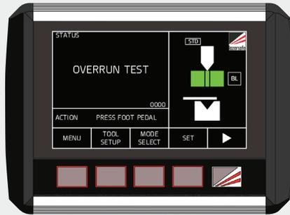
On start-up, the system initiates an automatic overrun test to check the machine stopping performance.
