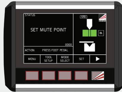
1. Place the flat part or sample material on the die (the same thickness as part to be formed).
