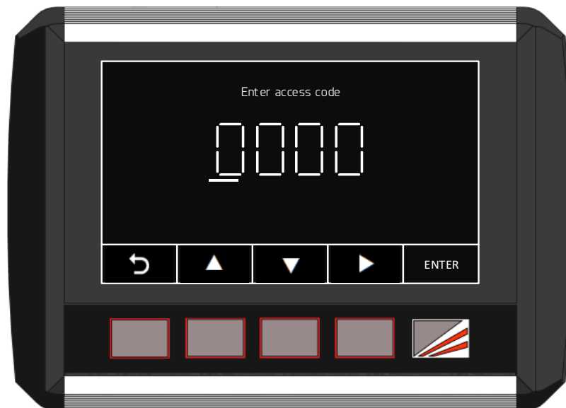
Figure 8-4: Supervisor Menu Access Screen
